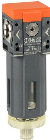
Metal Work Syntesi Size 1 pneumatic filter, particulate and moisture separation, 3/8in female NPT inlet(s), 3/8in female NPT outlet(s), manual/semi-automatic drain, clear technopolymer bowl, bowl guard.
