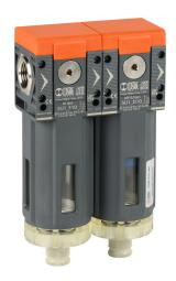
Metal Work Syntesi Size 1 pneumatic combination unit, filter-coalescing filter, 3/8in female NPT inlet(s), 3/8in female NPT outlet(s), clear technopolymer bowl, manual/semi-automatic drain.
