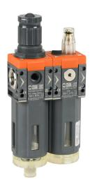
Metal Work Syntesi Size 1 pneumatic combination unit, filter-regulator-lubricator, 3/8in female NPT inlet(s), 3/8in female NPT outlet(s), 0 to 120 psig range, clear technopolymer bowl, manual/semi-automatic drain.
