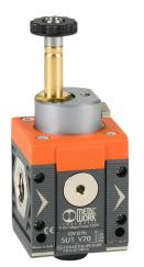
Metal Work shut-off valve, 3-port (3-way), 2-position, single solenoid spring return, N.C., 1/4in female NPT inlet(s), 1/4in female NPT outlet(s), G1/8 female BSPP exhaust(s), Cv=1.5. For use with Syntesi Size 1 air prep components.
