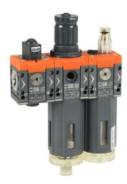
Metal Work Syntesi Size 1 pneumatic combination unit, valve-filter-regulator-lubricator, 1/4in female NPT inlet(s), 1/4in female NPT outlet(s), 0 to 120 psig range, clear technopolymer bowl, manual/semi-automatic drain, manual shutoff valve.
