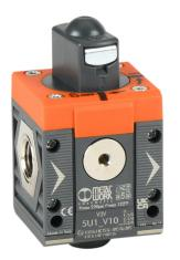
Metal Work shut-off valve, 3-port (3-way), 2-position, twist, N.C., 1/4in female NPT inlet(s), 1/4in female NPT outlet(s), G1/8 female BSPP exhaust(s), Cv=1.5. For use with Syntesi Size 1 air prep components.
