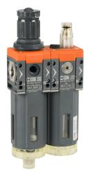
Metal Work Syntesi Size 1 pneumatic combination unit, filterregulator-lubricator, 1/4in female NPT inlet(s), 1/4in female NPT outlet(s), 0 to 120 psig range, clear technopolymer bowl, manual/ semi-automatic drain.
