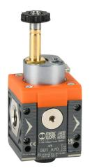
Metal Work soft start valve, 3-port (3-way), 2-position, single solenoid spring return, N.C., 1/4in female NPT inlet(s), 1/4in female NPT outlet(s), G1/8 female BSPP exhaust(s), Cv=1.5. For use with Syntesi Size 1 air prep components.
