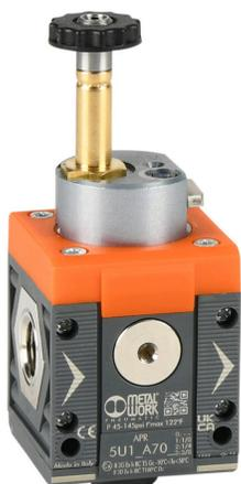
Metal Work soft start valve, 3-port (3-way), 2-position, single solenoid spring return, N.C., 1/4in female NPT inlet(s), 1/4in female NPT outlet(s), G1/8 female BSPP exhaust(s), Cv=1.5. For use with Syntesi Size 1 air prep components.
