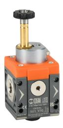
Metal Work shut-off valve, 3-port (3-way), 2-position, single solenoid spring return, N.C., 1/8in female NPT inlet(s), 1/8in female NPT outlet(s), G1/8 female BSPP exhaust(s), Cv=1.2. For use with Syntesi Size 1 air prep components.
