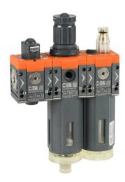
Metal Work Syntesi Size 1 pneumatic combination unit, valve-filter-regulator-lubricator, 1/8in female NPT inlet(s), 1/8in female NPT outlet(s), 0 to 120 psig range, clear technopolymer bowl, manual/semi-automatic drain, manual shutoff valve.
