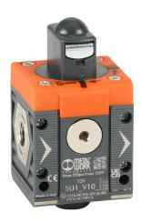
Metal Work shut-off valve, 3-port (3-way), 2-position, twist, N.C., 1/8in female NPT inlet(s), 1/8in female NPT outlet(s), G1/8 female BSPP exhaust(s), Cv=1.2. For use with Syntesi Size 1 air prep components.
