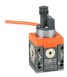
Metal Work pressure switch, air, 1/8in female NPT process connection, 7.5 to 145 psi set point, N.O./N.C. complementary, 2m 3-wire cable. For use with Syntesi Size 1 air prep components.
