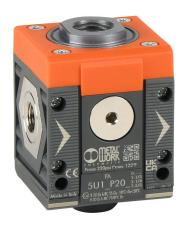
Metal Work pneumatic distribution block, 1/8in female NPT inlet(s), (1) 1/4in female NPT and (2) 1/8in female NPT outlet(s). For use with Syntesi Size 1 air prep components.
