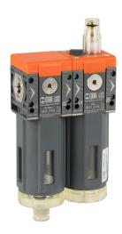
Metal Work Syntesi Size 1 pneumatic combination unit, filter-lubricator, 1/8in female NPT inlet(s), 1/8in female NPT outlet(s), clear technopolymer bowl, manual/semi-automatic drain.
