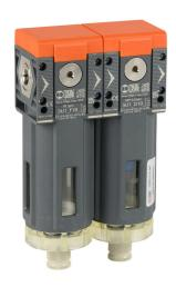
Metal Work Syntesi Size 1 pneumatic combination unit, filter-coalescing filter, 1/8in female NPT inlet(s), 1/8in female NPT outlet(s), clear technopolymer bowl, manual/semi-automatic drain.
