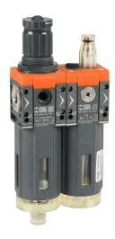
Metal Work Syntesi Size 1 pneumatic combination unit, filter-regulator-lubricator, 1/8in female NPT inlet(s), 1/8in female NPT outlet(s), 0 to 120 psig range, clear technopolymer bowl, manual/semi-automatic drain.
