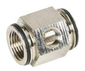
Metal Work air distribution block, 3/8in female NPT inlet(s), (1) 3/8in female NPT and (2) 1/8in female NPT outlet(s). For use with Syntesi Size 1 air prep components.
