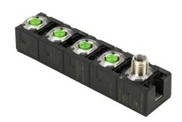
Murrelektronik IO-Link hub, up to (4) temperature input channel(s), (4) 5-pin M12 A-coded port(s), RTD, 24-bit, IO-Link v1.1.2 (compatible with v1.1.3), IO-Link Class A Device, IP65, IP67 and IP68. Requires IO-Link master.
