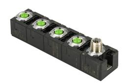
Murrelektronik IO-Link hub, up to (4) analog input channel(s), (4) 5-pin M12 A-coded port(s), current/voltage, 24-bit, IO-Link v1.1.2 (compatible with v1.1.3), IO-Link Class A Device, IP65, IP67 and IP68. Requires IO-Link master.
