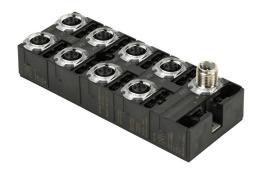
Murrelektronik IO-Link hub, up to (16) discrete I/O points, (8) 5-pin M12 A-coded ports, 24 VDC, IO-Link v1.1.2 (compatible with v1.1.3), IO-Link Class B Device, 4A, 2A/port, IP68. Requires IO-Link master.
