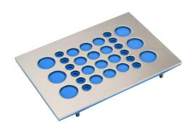
Murrplastik FDA cablequick KDP series cable entry system frame, stainless steel frame, 132x82mm frame, (12) 3.5-6.2mm, (12) 6-10mm, (6) 9-14mm opening(s), IP65.
