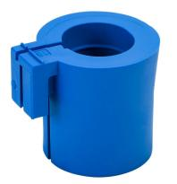
Murrplastik KDT/X-FDA series medium grommet, 1 opening(s), TPE, blue, accepts 15-16mm diameter cable. Package of 4. For use with Murrplastik KDL/H-VA-FDA series cable entry system frame.
