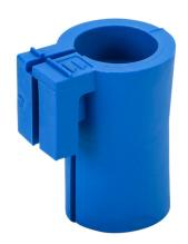
Murrplastik KDT/X-FDA series small grommet, 1 opening(s), TPE, blue, accepts 11-12mm diameter cable. Package of 4. For use with Murrplastik KDL/H-VA-FDA series cable entry system frame.
