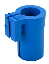
Murrplastik KDT/X-FDA series small grommet, 1 opening(s), TPE, blue, accepts 10-11mm diameter cable. Package of 4. For use with Murrplastik KDL/H-VA-FDA series cable entry system frame.
