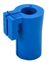
Murrplastik KDT/X-FDA series small grommet, 1 opening(s), TPE, blue, accepts 8-9mm diameter cable. Package of 4. For use with Murrplastik KDL/H-VA-FDA series cable entry system frame.
