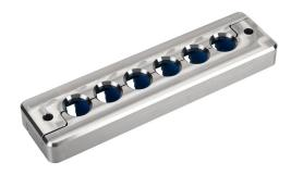
Murrplastik KDL/H-VA-FDA series cable entry system frame, stainless steel frame, 112x17mm frame, (6) small opening(s), IP69K. Requires (6) Murrplastik KDT/X-FDA series small grommets.
