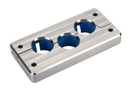
Murrplastik KDL/H-VA-FDA series cable entry system frame, stainless steel frame, 16-pin frame, (3) medium opening(s), IP69K. Requires (3) Murrplastik KDT/X-FDA series medium grommets.
