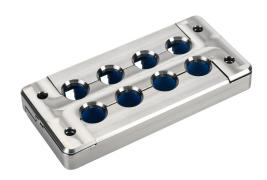
Murrplastik KDL/H-VA-FDA series cable entry system frame, stainless steel frame, 16-pin frame, (8) small opening(s), IP69K. Requires (8) Murrplastik KDT/X-FDA series small grommets.
