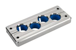
Murrplastik KDL/H-VA-FDA series cable entry system frame, stainless steel frame, 24-pin frame, (4) medium opening(s), IP69K. Requires (4) Murrplastik KDT/X-FDA series medium grommets.
