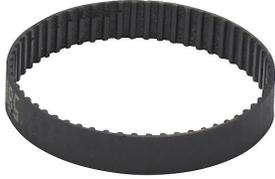
SureMotion timing belt, 0.08in MXL pitch, 1/4in wide, 58 tooth, 4.6in pitch length (circumference), neoprene, fiberglass reinforced. Package of 3.
