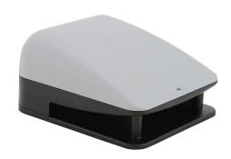
WERMA audible signal horn, 105 dB at 1m, 100 Hz tone frequency, continuous tone(s), 115 VAC, wall mount, ABS plastic housing, light gray, IP65.
