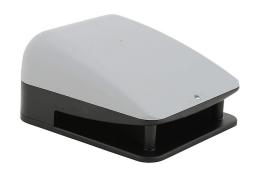
WERMA audible signal horn, 105 dB at 1m, 100 Hz tone frequency, continuous tone(s), 115 VAC, wall mount, ABS plastic housing, light gray, IP65.
