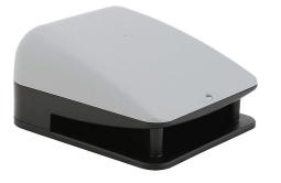
WERMA audible signal horn, 105 dB at 1m, 100 Hz tone frequency, continuous tone(s), 24 VDC, wall mount, ABS plastic housing, light gray, IP65.
