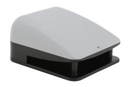
WERMA audible signal horn, 105 dB at 1m, 100 Hz tone frequency, continuous tone(s), 24 VDC, wall mount, ABS plastic housing, light gray, IP65.
