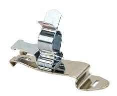
Murrplastik SCFZ-EMV series EMC shield cable clip, accepts 0.43-0.63in diameter cable, 35mm DIN rail mount, with strain relief, zinc plated spring steel. Package of 5.
