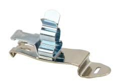
Murrplastik SCFZ-EMV series EMC shield cable clip, accepts 0.31-0.43in diameter cable, 35mm DIN rail mount, with strain relief, zinc plated spring steel. Package of 5.
