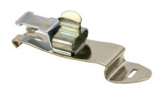
Murrplastik SCFZ-EMV series EMC shield cable clip, accepts 0.06-0.12in diameter cable, 35mm DIN rail mount, with strain relief, zinc plated spring steel. Package of 5.
