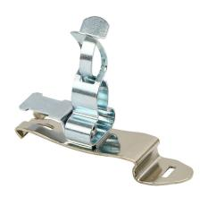
Murrplastik MSCFZ-EMV series EMC shield cable clip, accepts 0.28-0.71in diameter cable, 35mm DIN rail mount, with strain relief, zinc plated spring steel. Package of 5.
