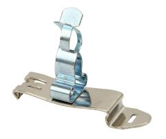
Murrplastik MSCF-EMV series EMC shield cable clip, accepts 0.28-0.71in diameter cable, 35mm DIN rail mount, zinc plated spring steel. Package of 5.
