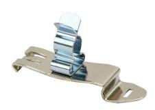
Murrplastik SCF-EMV series EMC shield cable clip, accepts 0.31-0.43in diameter cable, 35mm DIN rail mount, zinc plated spring steel. Package of 5.
