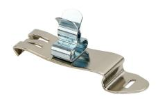
Murrplastik SCF-EMV series EMC shield cable clip, accepts 0.12-0.24in diameter cable, 35mm DIN rail mount, zinc plated spring steel. Package of 5.
