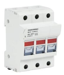
Socomec modular fuse holder, with indicator, accepts Class CC fuses, 30A, 600 VAC, 3-pole, 18-8 AWG copper only, pressure plate, 35mm DIN rail mount. Package of 4.
