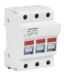
Socomec modular fuse holder, with indicator, accepts Class CC fuses, 30A, 600 VAC, 3-pole, 18-8 AWG copper only, pressure plate, 35mm DIN rail mount.
