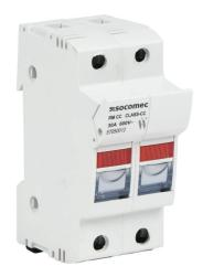
Socomec modular fuse holder, with indicator, accepts Class CC fuses, 30A, 600 VAC, 2-pole, 18-8 AWG copper only, pressure plate, 35mm DIN rail mount. Package of 6.
