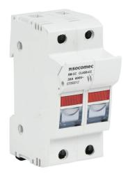
Socomec modular fuse holder, with indicator, accepts Class CC fuses, 30A, 600 VAC, 2-pole, 18-8 AWG copper only, pressure plate, 35mm DIN rail mount.
