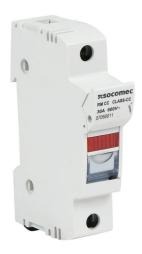
Socomec modular fuse holder, with indicator, accepts Class CC fuses, 30A, 600 VAC, 1-pole, 18-8 AWG copper only, pressure plate, 35mm DIN rail mount. Package of 12.
