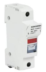
Socomec modular fuse holder, with indicator, accepts Class CC fuses, 30A, 600 VAC, 1-pole, 18-8 AWG copper only, pressure plate, 35mm DIN rail mount.
