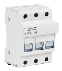
Socomec modular fuse holder, accepts Class CC fuses, 30A, 600 VAC, 3-pole, 18-8 AWG copper only, pressure plate, 35mm DIN rail mount. Package of 4.
