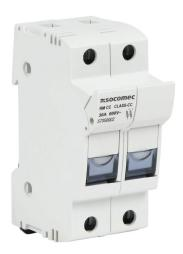
Socomec modular fuse holder, accepts Class CC fuses, 30A, 600 VAC, 2-pole, 18-8 AWG copper only, pressure plate, 35mm DIN rail mount. Package of 6.
