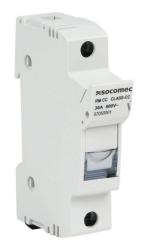
Socomec modular fuse holder, accepts Class CC fuses, 30A, 600 VAC, 1-pole, 18-8 AWG copper only, pressure plate, 35mm DIN rail mount. Package of 12.
