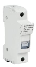
Socomec modular fuse holder, accepts Class CC fuses, 30A, 600 VAC, 1-pole, 18-8 AWG copper only, pressure plate, 35mm DIN rail mount.
