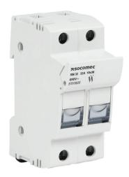
Socomec modular fuse holder, accepts Class Midget fuses, 30A, 750 VAC, 2-pole, 18-8 AWG copper only, pressure plate, 35mm DIN rail mount. Package of 6.
